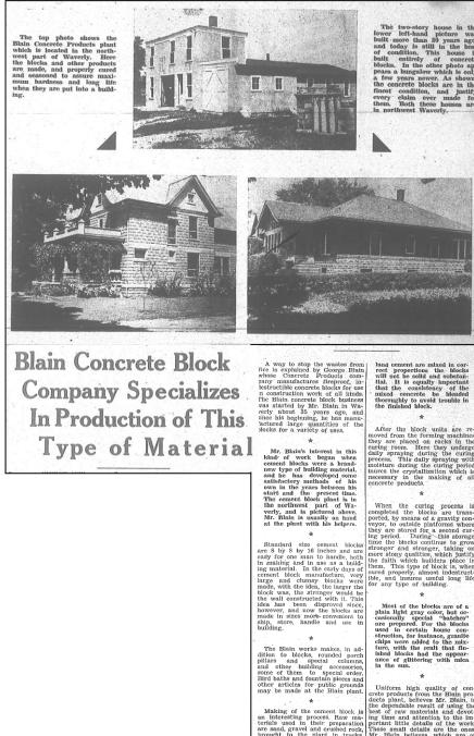
brought to the plant in trucka. These raw materials are combined with Portland cement and clean water in an open mixer especially designed to meet the particular replants. After the ingredients are mixed thoroughly, the mixture is placed in sturdily-constructed block machines and tamped repeatedly with automatic tampers to insure smoothness.
