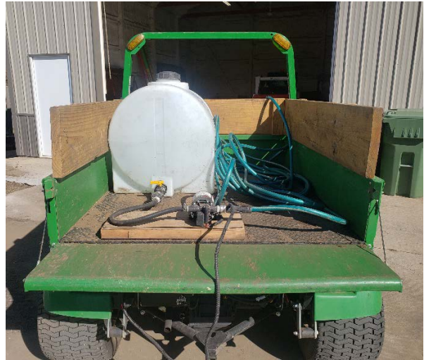
(New water tank/pump setup)
